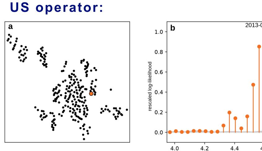
The algorithm consistently points to the same candidate source in a similar frequency range even for time series collected over two time periods separated by almost a month (March 2013 vs. April 2013).
