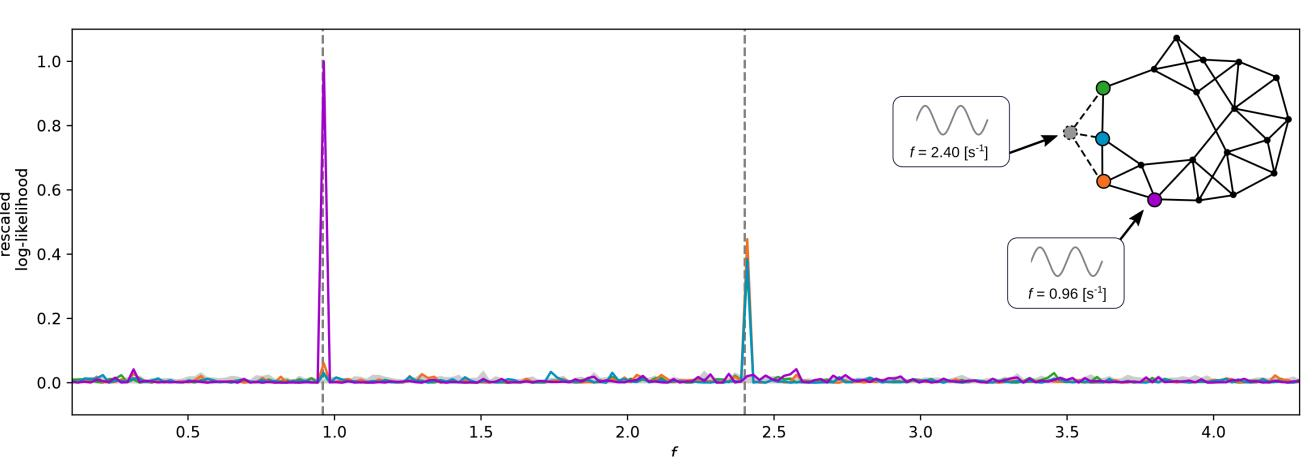
Conclusions Solely based on time-series measurements of voltage angles and frequencies our algorithm is able to identify the forcing frequency and locate the source. A relaxed version of the algorithm makes it scalable to large systems (see Ref.[1]).
