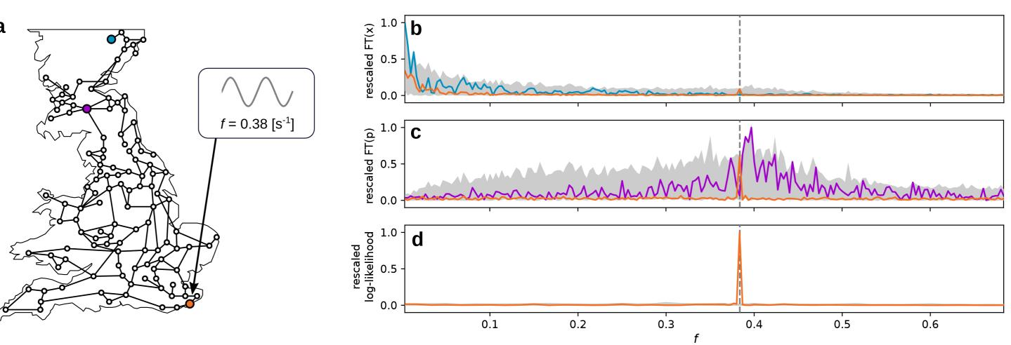
Outcome of the Fourier transform of the positions and velocities at each bus and of the optimization of the log-likelihood for a model of the UK power grid.
